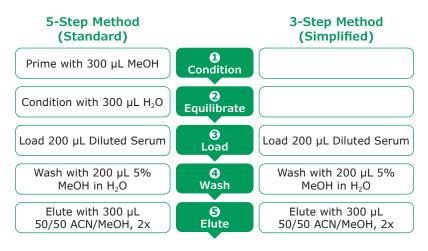
**Figure 1.** General processing of samples (serum 1:1 diluted) with Supel<sup>TM</sup> Swift HLB cartridges (30 mg/1 mL) using a 5-step method and a 3-step method
