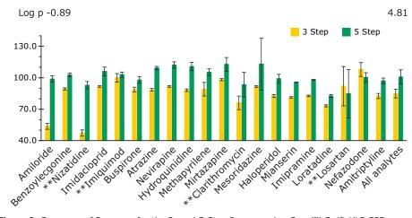
Figure 2: Summary of Recovery for the 3- and 5-Step Process using Supel™ Swift HLB SPE cartridges. Analytes are ordered by increasing log P values.
