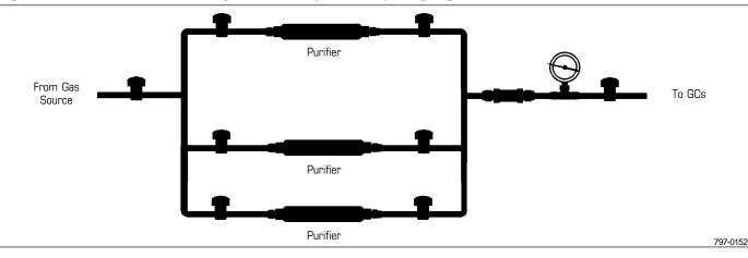
removal by including a High Capacity Heated Purifier for each bench of chromatographs, yet accommodates the lower maximum flow allowed by the heated purifier.
