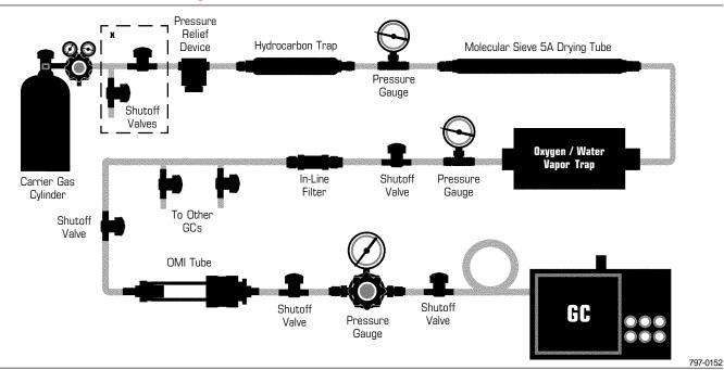
T197918 BIT and water can be overwhelmed by these high levels of contaminants; some oxygen/water traps even could be damaged. For example, an indicating purifier or heated purifier could overheat, possibly releasing previously trapped oxygen and water. Worse, overheating could break down the catalyst particles or coated beads in the purifier, generating contaminating breakdown products and/or possibly plugging the purifier or greatly increasing the back pressure.
