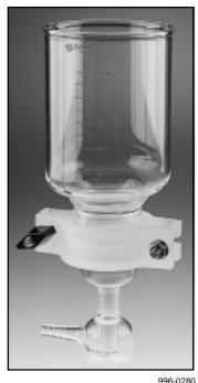
The ENVI-Disk Clamp is for use with standard glass filtration apparatus (47mm or 90mm) to create a better seal for eliminating leaks when using SPE extraction disks or filtering HPLC mobile phase solvents.
