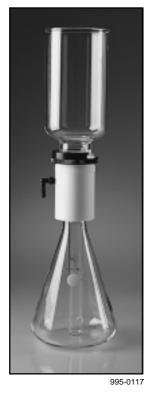
The ENVI-Disk Holder is designed to be used with 47mm ENVI-Disk solid phase extraction disks. The unit consists of a 1-liter sample funnel, a threaded screw clamp, a Teflon disk support, and a Teflon filter base/ adapter with a vacuum attachment fitting. The filter base fits onto any standard 1-liter flask that has a 40/35 tapered ground glass neck. A 25 x 250mm test tube is used with the flask to collect disk eluates.
