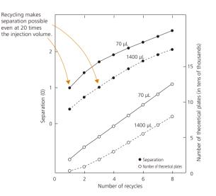
Example in Which Recycle Separation with a Semi-Preparative GPC Column Improves the Preparative Processing Speed (LC-20AR Recycle System)
