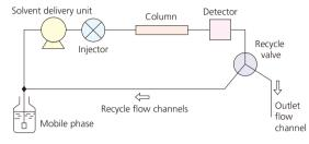
Flow Channels Used for Closed Loop Recycling
