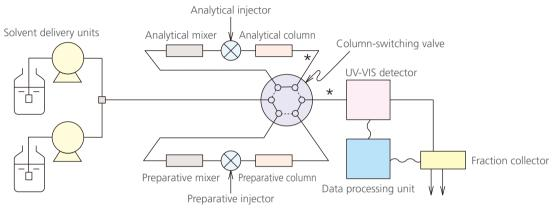
\* Analytical samples pass through piping created with 0.3 mm inner diameter tubes.
