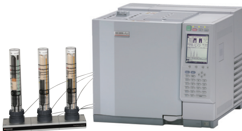
Example of Shimadzu Gas Filter Kit for GC-FID
