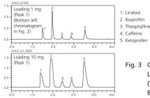
Fig. 3 Chromatogram Obtained during Loading Investigation (Nexera UC) (Top: Before loading increase. 2 µL injected, Bottom: After loading increase. 20 µL injected)
