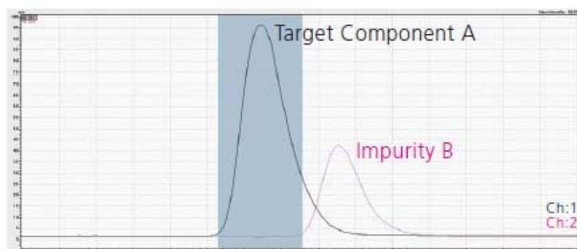
High Purity Recovery of Target Component A (Using two MS signals as triggers)
