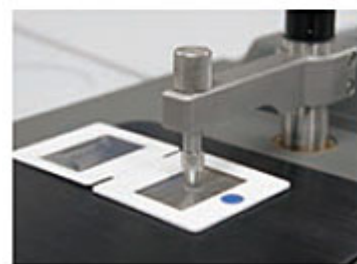
Measurement with FTIR
