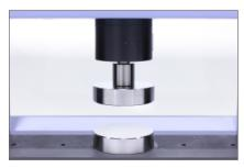
Upper and lower compression plates should be mounted parallel
