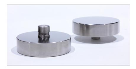
Fixed compression plates, or platens as they are otherwise known, are versatile testing accessories, applicable to compression and cycle testing a diverse range of materials and finished products. Hardened faces, surface hardness of 60 on the Rockwell HRC scale, ensure minimal wear, preserving surface smoothness.
