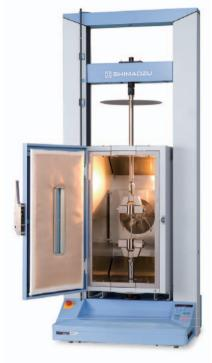
AGS-10kNXD + Screw Type Flat Grips + Compact Thermostatic Chamber TCE series
