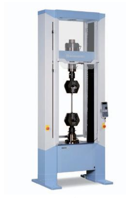
AGS-300kNX + 300kN Non-Shift Wedge Type Grips
