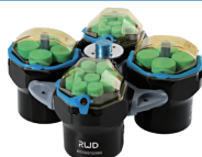
Self-locking swing-out rotor
