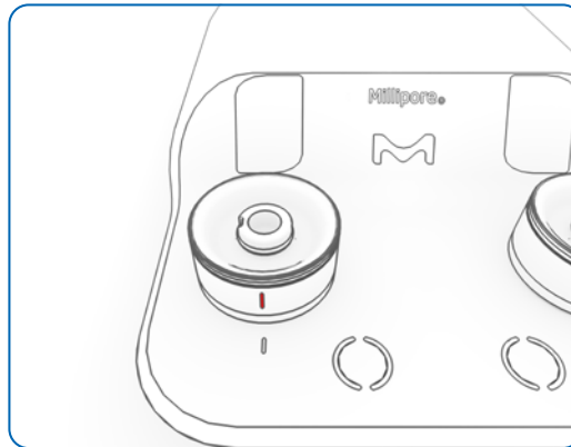
Figure 33: The sign on a locked head is aligned with the one on the pump body
