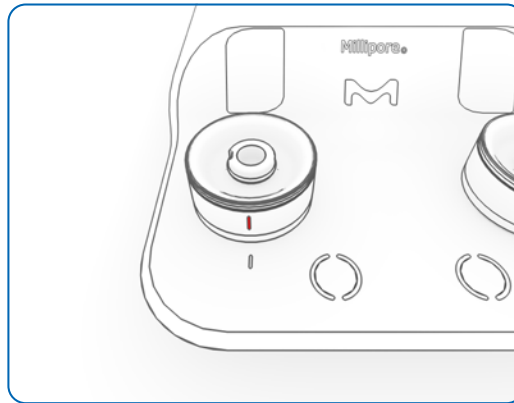
Figure 11: The sign on a locked head is aligned with the one on the pump body
