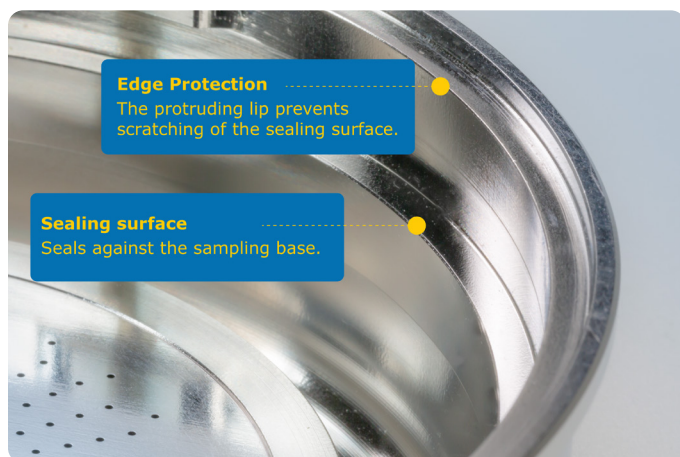
Figure 4: Stainless steel perforated lid (upside down). The edge protection prevents scratching of the sealing surface which would lead to aspirating air through the gap.
