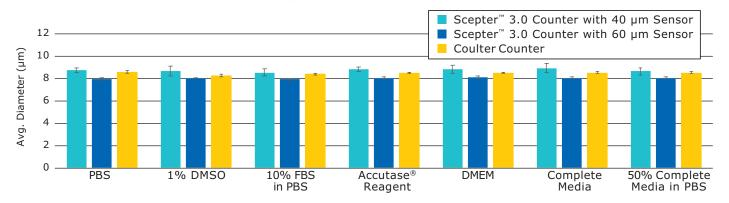
Polystyrene beads of known diameter (8  $\mu$ m) suspended in various cell culture buffers and reagents were measured using the Scepter<sup>TM</sup> 3.0 Cell Counter with both 40  $\mu$ m and 60  $\mu$ m sensors. Results are compared to the same counts obtained with a Coulter Counter Z2<sup>TM</sup> Instrument equipped with 100  $\mu$ m aperture. Data are from three measurements per sample.
