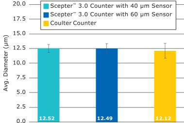
Jurkat cells were measured to test accuracy and reproducibility of cell size measurements using the Scepter  $^{\text{TM}}$  3.0 Cell Counter with both 40  $\mu m$  and 60  $\mu m$  sensors. Results are compared to the same measurement obtained with a Coulter Counter Z2  $^{\text{TM}}$  Instrument equipped with 100  $\mu m$  aperture. Data are from five measurements per sample.
