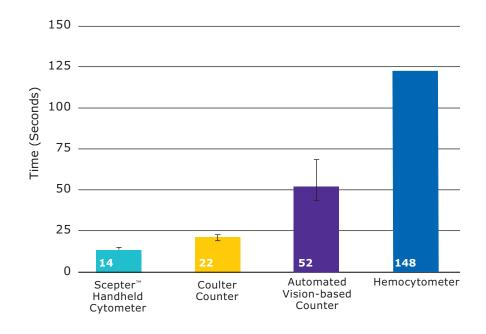
The time required to perform cell counts using various methods was compared using a sample concentration of 500,000 cells/mL. Scepter™ counting (14 seconds on average, using the 60 µm sensor) is significantly faster than other counting methods. Using the 40 µm sensor, Scepter™ counts are complete within 25 seconds, on average (data not shown).
