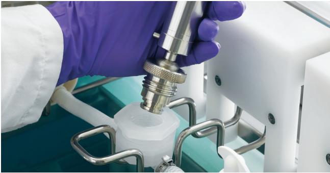
Figure 3. The innovative low dead volume t-connector protects the process fluid from contamination.
