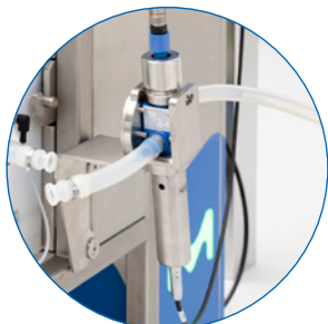
Pre-column instrumentation for conductivity and pH measurement
