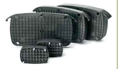
Millistak+® CR depth filter media is formulated with carbon retained in a rigid structure by a cellulose matrix. These materials, combined with a state-of-the-art manufacturing process, create a tortuous flow path that ensures increased contact with the surface and pores of the activated carbon, for optimum impurity adsorption.
