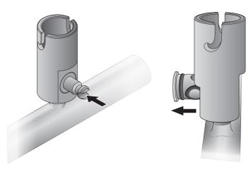
4. Remove each of the 3 O-rings from the valve by placing the tips of the filter forceps into the small notch near each O-ring. Grasp the ring in the tips of the forceps and remove it.
