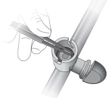
4. Clean the O-ring and the filtration head support using a nonwoven wipe moistened with one of the products listed in the recommended cleaning agents list in this section.
