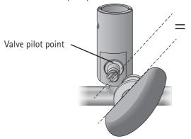
15. Keeping the end of the valve in place, push the valve button onto the valve pilot point until it clicks.
