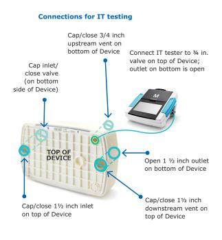
Figure 1. Schematic showing connections to Viresolve Pro<sup>®</sup> Magnus Device during integrity testing. The same procedures on automated testers are performed for both pre- and post-use integrity tests. After wetting and firmware checking, the liquid held up in the filter is cleared before a pre-pressurization period to ensure that liquid downstream of the filter is removed.
